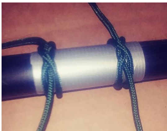
Duct tape patch with constrictor knots
