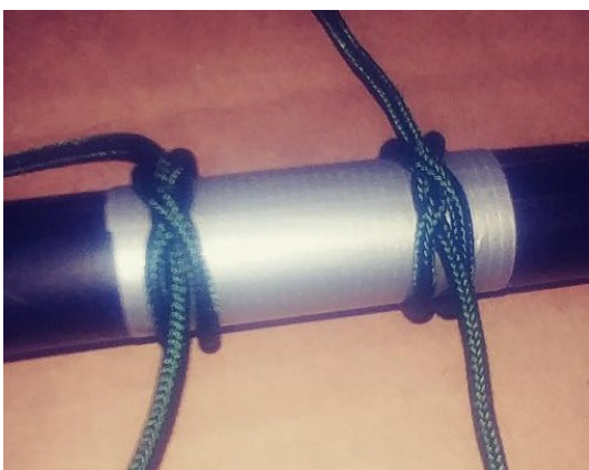
Duct tape patch with constrictor knots
